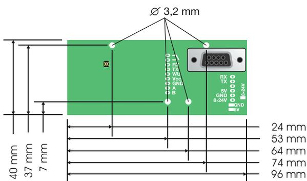
figure 4 - Dimensions of the circuit board
