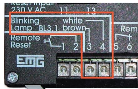
figure 1 - example of blinking lamp connector (can be also used for BL4.1 and BL6)
