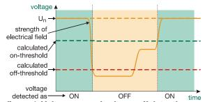
figure 4: Voltage-on and voltage-off detection
